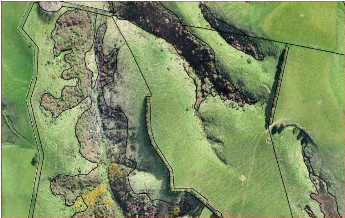
Photo 1: Drone mapping survey. Photogrammetry, utilising overlapping images processed into georeferenced true to scale ortho photo to use in SFL GIS/Mapping system
